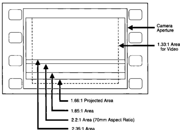
**Illustration 8 - Super 35/Super Techniscope Common Topline**
