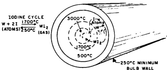
Figure 14. Diagram of Halogen Cycle within lamp.
