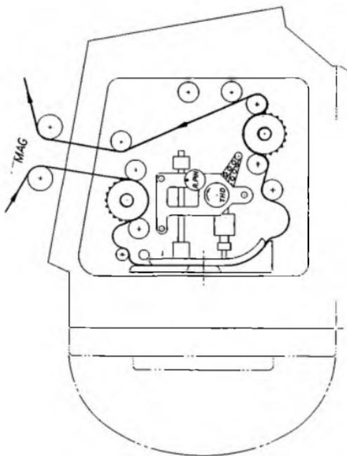
This camera, designed in conjunction with Wilcam, is intended to meet the exacting needs of Showscan cinematography (60 fps) but operates at conventional speeds as well. Photographed aperture is standard 5-perf 65mm (2.072" x 0.906").
