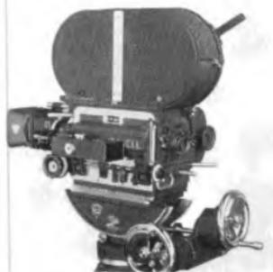
The NC camera differs from the "standard" model in that it uses a mechanically different and quieter movement and has other features which make it quieter. NC, BNC, FC, BFC are rack-over models. NCR, BNCR are reflex models. NC model has a four-lens turret, the others a single lens mount. B models are blimped versions.
