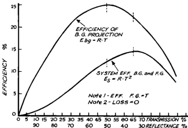
Figure 2. Front projection mirror; transmission/reflection ratio and efficiency.
