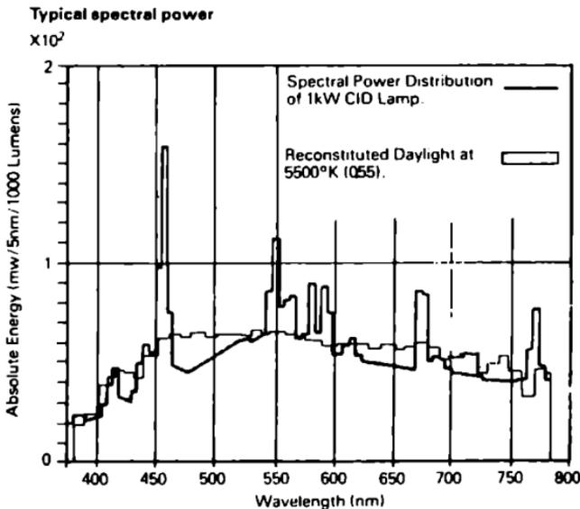
Figure 27. Typical spectral power distribution for CID lamps.
