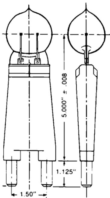
Figure 26. 2500-W compact iodide daylight (CID).
