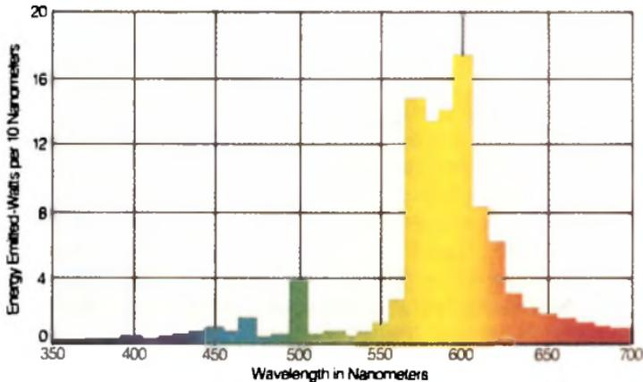
Figure 41. Spectral power distribution of 400-W sodium lamp, similar to types known as Lucelox or Lumalux.
