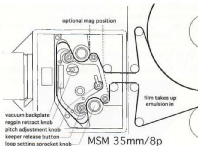
camlock secures the mag in running position and switches power to the motor and heater contacts in the magfoot. Expanding core hubs have integral DC servomotors controlled by film tension in both directions, with soft startup to eliminate slack. Tightwind rollers guide film winding for smooth solid rolls at any camera angle. Non-contact light traps feature infrared end-of-film sensors.
