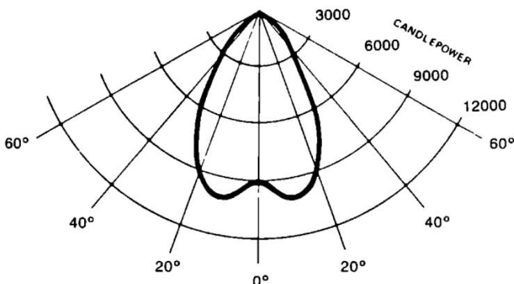
Figure 8. Luminaire intensity distribution—polar.
