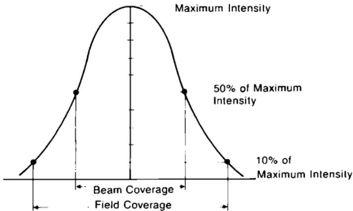
Figure 9. Definition of intensity distribution curves.
