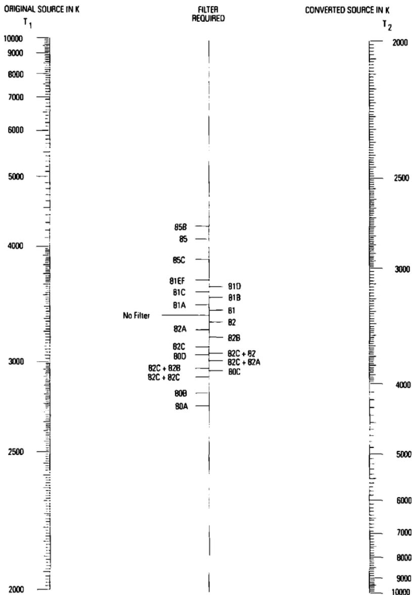
The nomograph can be used to find the approximate filter for a particular conversion by placing a straightedge from an original source ( $T_1$ ) to a second source ( $T_2$ ). The approximate filter can be found on the center line.
