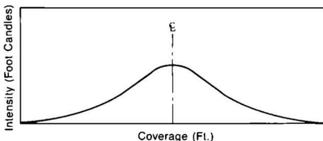
Figure 55. Characteristic intensity curve of tungsten-halogen floodlight (broad) (horizontal axis).
