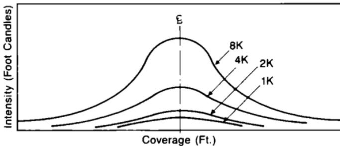
Figure 59. Characteristic intensity curves of "soft" lights.
