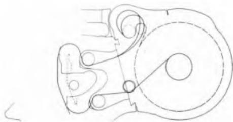
**Movement:** 35BL-1 through BL-4 cameras feature dual-pin registration and dual pull-down claws that advance the film through a fixed-gap film channel. The 35BL-4s has a technologically advanced movement that includes an adjustable pitch control. Aperture plates and ground glasses for all aspect ratios are interchangeable between all 35BL models.
