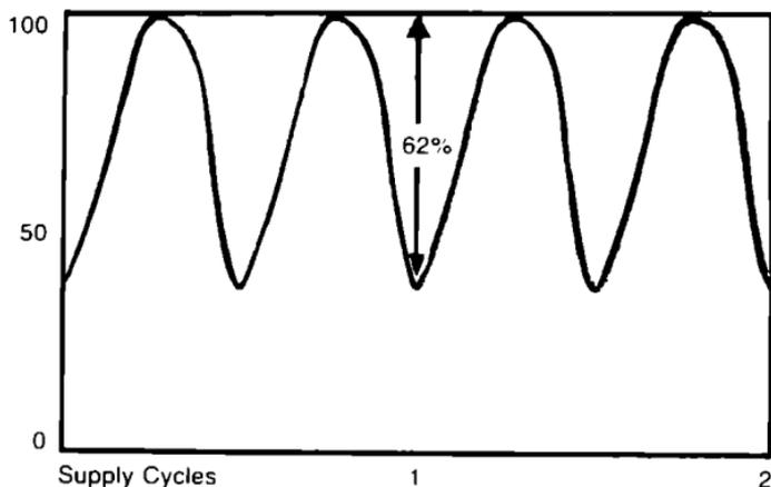
Figure 44. Waveform for a 1000-W CSI lamp.
