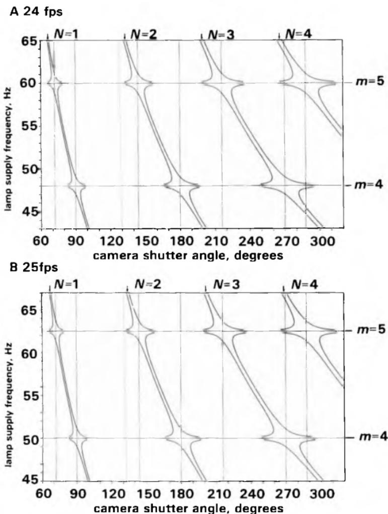
Figure 45A and B. Contours of safe lamp supply frequencies for one ripple ratio value.  $m$  is the nearest whole number to the number of ripple cycles in the camera frame period.  $N$  is the nearest whole number to the number of ripple cycles in the exposure interval.
