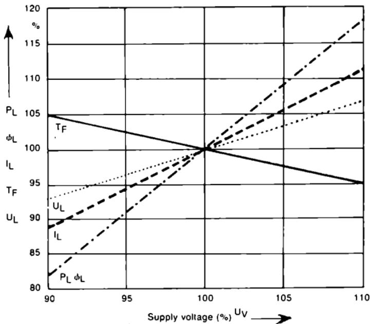
Figure 22. HMI 2500-W power consumption  $P_L$ , luminous flux  $\phi_L$ , current intensity  $I_L$ , nearest color temperature  $T_F$ , and operating voltage  $U_L$  (relative values), as a function of the supply voltage  $U_v$ .
