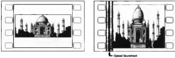
**Illustration 10 - Super 35 Aspect Ratio 2.35:1. Above Left: The scene as it appears on the negative, positioned within the FULL aperture frame. Above Right: The scene as it appears on a print for projection, after being blown up & "squeezed" to make room for the optical soundtrack.**
