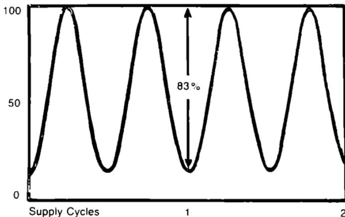
Figure 43. Waveform for an HMI lamp.
