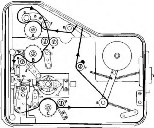
35mm highspeed (300 fps) pin-registered reflex camera.
