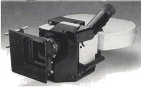
**Movement:** MSM Monoblock high-speed, triple register pins, claw engages four perfs. Shrinkage adjustment changes both stroke and entry position. Indexable loop-setting sprockets have independent locking keeper rollers. Vacuum backplate assures film plane accuracy, removes without tools for cleaning. Aperture and movement remove easily for cleaning and lubrication. Aperture size 1.485" wide x .992" high. Frame-rates from time-lapse to 72 fps forward, to 30 fps reverse.
