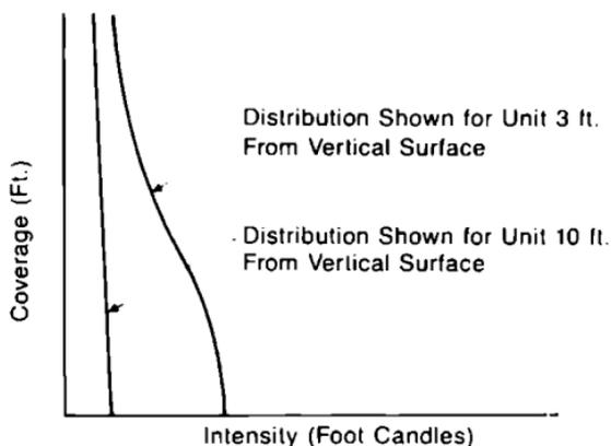
Figure 57. Characteristic intensity curve for cyclorama light.
