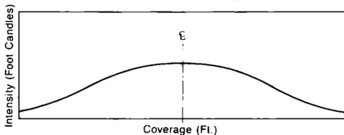
Figure 56. Characteristic intensity curve of "mini" floodlight (horizontal axis).
