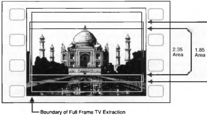
**Illustration 7 - Standard Super 35/Super Techniscope**
