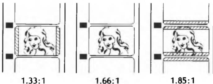
The aspect ratio of the picture frame of a Super 16mm negative is 1.66:1.
