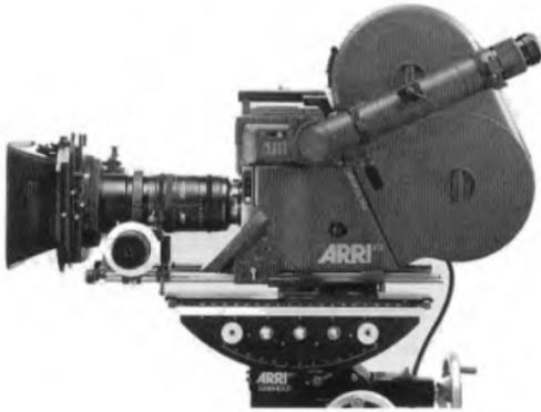
**Movement:** The 765 uses advanced microprocessor control technology to link two quartz-controlled DC motors in a direct drive configuration to control shutter and film transport. No belts or mechanical couplings are used in the drive system. Dual registration pins, triple-pin pull-down claws and user-adjustable pitch control assure image quality to optical printer standards.
