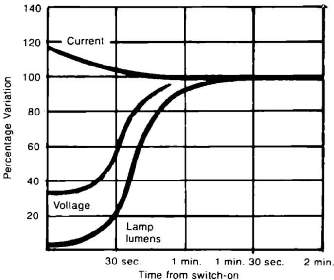
Figure 28. Transient characteristics of lamp from switch-on.
