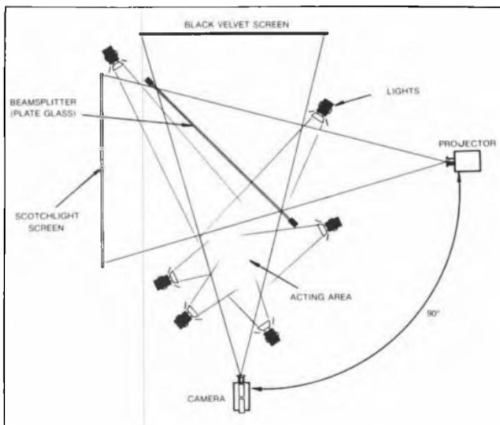
Figure 1. Diagram of reverse front projection.
