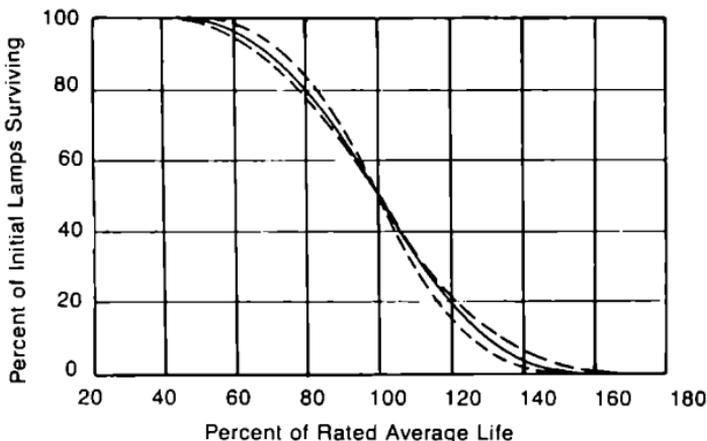
Figure 19. Life expectancy curve for tungsten filament lamps.
