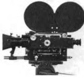
**Movement:** Single claw, single (or double for double system sound) registration pin. Adjustable stroke. Three sprockets. Removable aperture plate has built-in filter slot. Movement removable without losing timing. Speed range 16-64 fps. Alternate non-metallic and steel gears for quietness. Guides and locks interlocked with compartment door.
