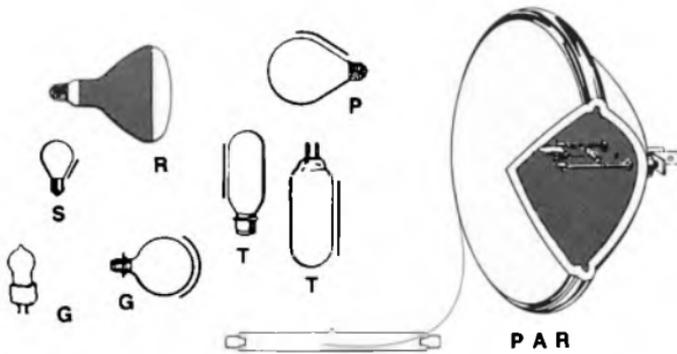
Figure 1. Lamp envelope configurations.
