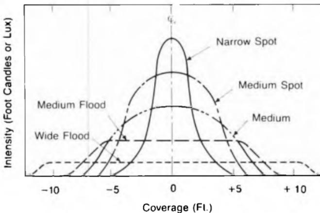
Figure 49. Characteristic intensity curve of Fresnel Spotlights.
