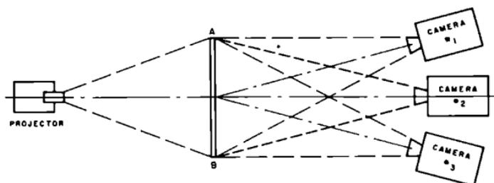
Camera and projector must be lined up so that the screen image is photographed with equal brilliance across its full width. Camera #2 will photograph screen "A-B" with even brilliance. Camera 1 will record the "B" side of the screen darker. Camera #3 will record the "A" side of the screen darker.
