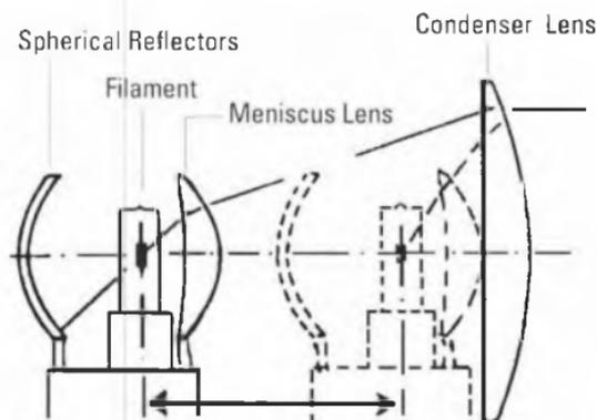
Figure 51. Dedolight Optical System.
