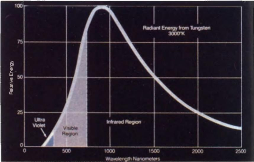
Figure 5. Spectral energy distribution for 1000-watt lamp with approximate color temperature of 3000 degrees K.
