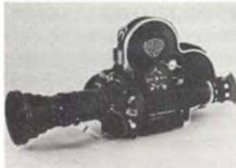
**Arriflex 16S/B:** Features pin-registered film transport system operating to 75 fps, 100-foot internal daylight film spool loading, with top-loading 400-foot magazine, reflex viewfinder system, divergent three lens-mount turret, and motor interchangeability.
