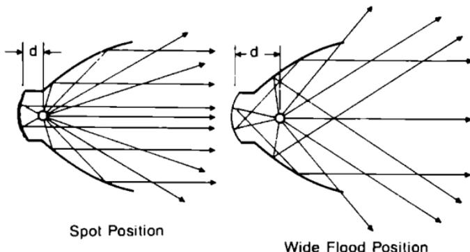
Figure 53. Optical system of non-lens spotlight (variable beam).
