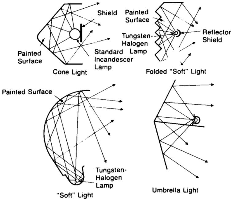
Figure 58. Optical system of various "soft" lights.
