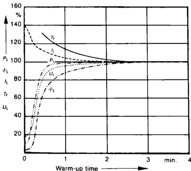
Figure 23. HMI 2500-W power consumption  $P_L$ , luminous flux  $O_L$ , current intensity  $I_L$ , nearest color temperature  $T_R$ , and operating voltage  $U_L$  (relative values), as a function of time after starting the cold lamp.
