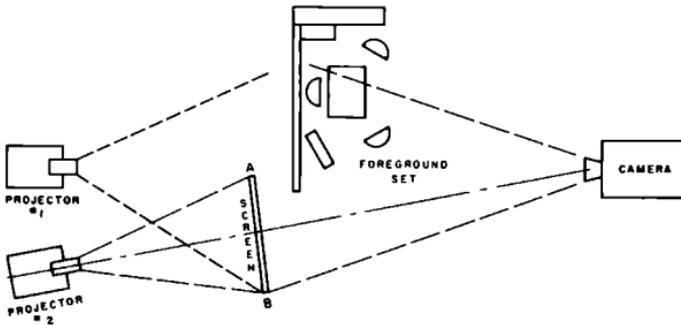
Camera and projector must be lined up when the camera is panned from a screen image on one side of a live set to the action on the opposite side. Projector #2 is correctly positioned. Projector #1 would result in a darker image on the "B" side of the screen.
