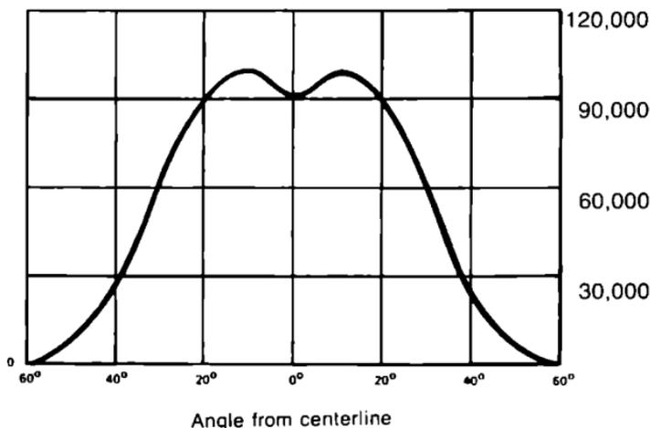
Figure 7. Luminaire intensity distribution—rectangular.
