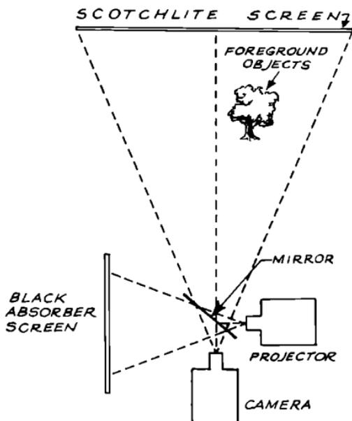
Figure 1. Arrangement of camera, projector, mirror and screen.
